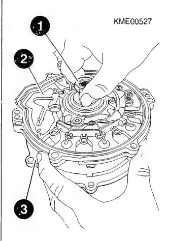
ASSEMBLING ALTERNATOR Assembling drive-end shield Secure drive-end shield (1) with housing connecting bolts (2). Fasten the 3 studs of the phase contacts (3). Use torque wrench. Tightening torques Housing attachment: 2,3...2,7 Nm 1.0...1.4 Nm Phase contacts: comm. avail. Torque wrench: TORX T20: comm. avail. TORX T25: comm. avail.
